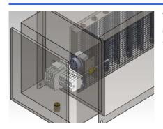
This range consists of wire heater mounted in galvanized steel rectangular duct and complete with:
